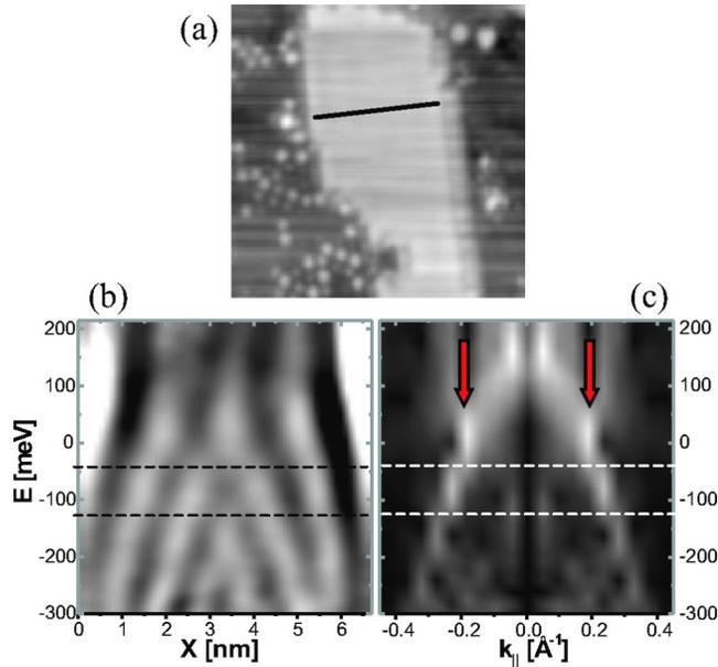
FIG. 3. (Color online) (a) Topographic image of an elongated resonator. Image size,  $15 \times 15 \text{ nm}^2$ ; sample bias,  $-500 \text{ mV}$ ; tunneling current,  $1.0 \text{ nA}$ . (b) LDOS as a function of energy  $E$  and position  $x$  along the line drawn in (a). (c) One-dimensional Fourier transform along the  $x$  axis of the data in (b). The actual wave-vector values have been divided by a factor of 2.
