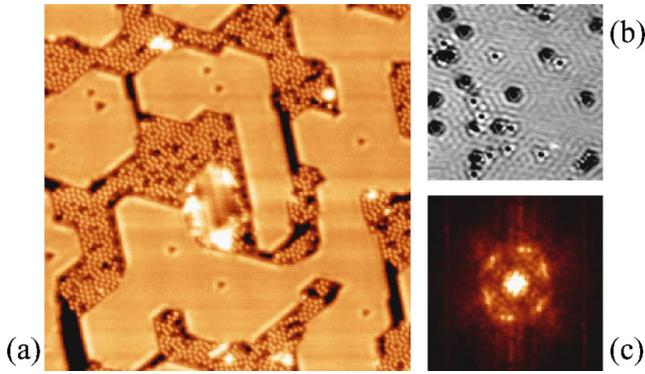
FIG. 1. (Color online) (a) Constant current image of a 0.5 ML Er deposit taken at 42 K. Size of the image,  $50 \times 50 \text{ nm}^2$ ; sample bias, +1.0 V; tunneling current, 1.0 nA. (b)  $40 \times 40 \text{ nm}^2$  constant current image of a 1.0 ML deposit taken at 40 K. Sample bias, -3 mV; tunneling current, 0.1 nA. (c) Fourier transform of (b). Size of the frame:  $10.1 \times 10.1 \text{ nm}^{-2}$  (the actual wave-vector values have been divided by a factor of 2).
